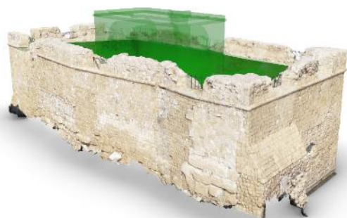
Figure 7. Paphos Castle seaside wall textured mesh in Rhinoceros software linked with the 3D Revit elements with green colour.
