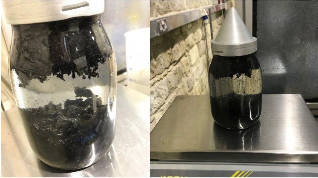
Figure 1 Measuring the Apparent Particle Density by EN 1097-6 : 2013
