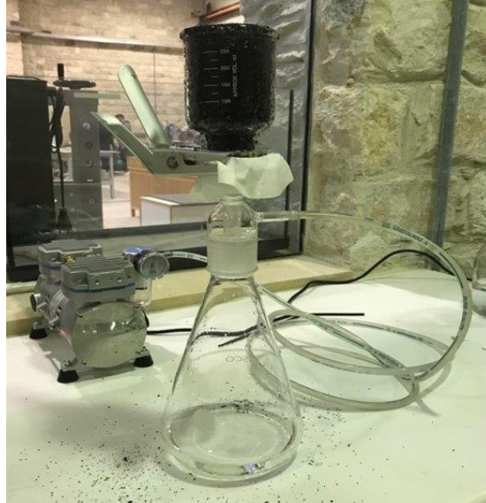
Figure 2 Water absorption of Lightweight Aggregate Test by EN 1097-6: 2013
