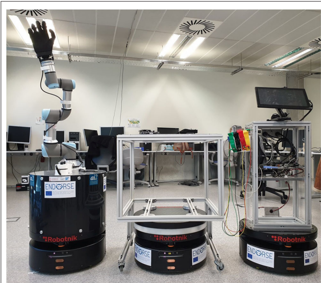
FIGURE 1 | ENDORSE project proof-of-concept mobile robotic fleet [http://www.endorse-project.eu/]. Robotnik's RB-1 robot is used with different, easily swappable, and mountable hardware modules. From left to right, a robotic arm (Universitat Politècnica de Valencia, Spain), a carrier component for logistic tasks (Robotnik, Spain), and an e-diagnostic module for vital signs acquisition (StreamVision, France) and communication to a cloud-based electronic health record (EHR) system (University of Cyprus, Cyprus).
