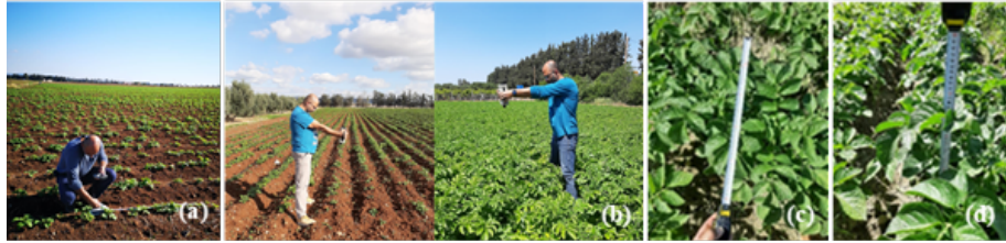
Fig. 4. (a) Potato: LAI data collection below canopy and inter row; (b) Potato: Data collection using a GER1500 spectroradiometer in potatoes during BBCH19 (left) and BBCH 39 (right); (c) Potato BBCH 38: 80% of plants meet between rows, measuring plant diameter
