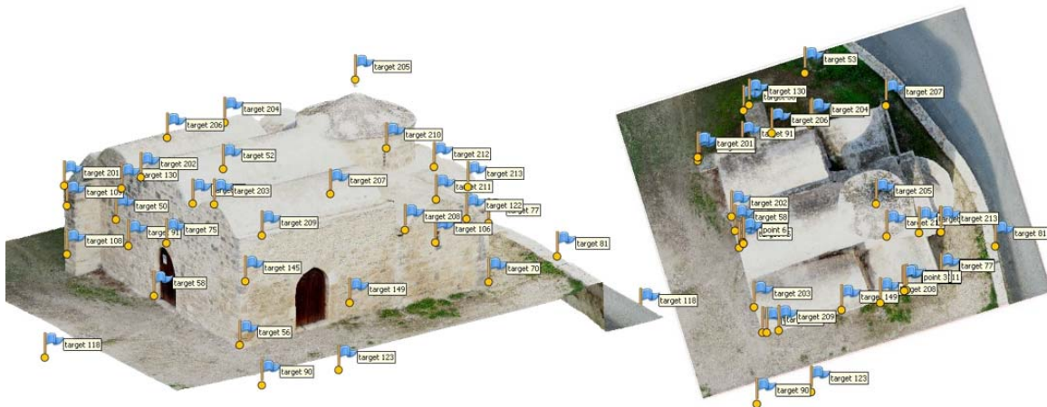
Figure 3: Ground control points with total station registration
