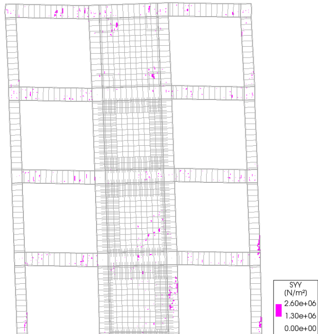
Figure 5.8: Tensile stress of 2.6MPa at 5.968seconds (maximum displacement of the frame in the west direction) at the east column of the frame
