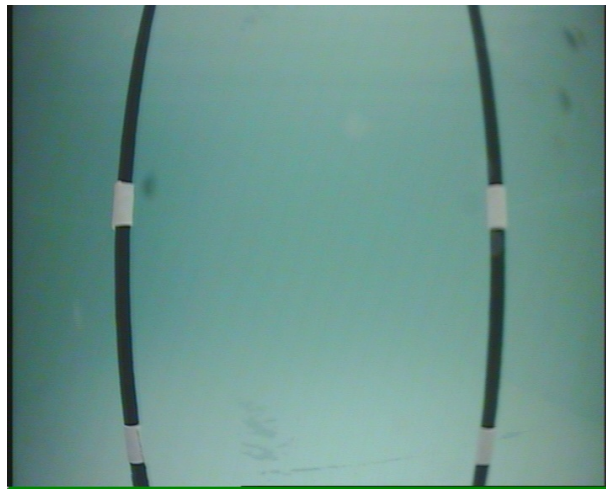
Figure 3.17: Targets fitted at 50mm apart on a plane 82mm from the dome base(Underwater)
