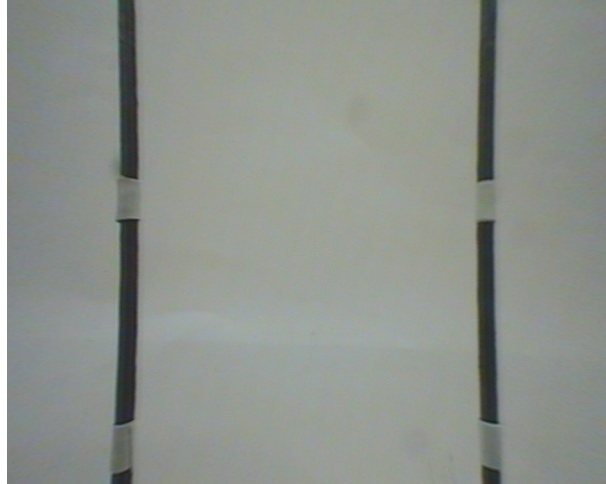
Figure 3.16: Targets fitted at 50mm apart on a plane 82mm from the dome base(Air)
