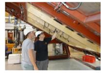
Fig.1. Large-scale laboratory wind-driven rain tightness testing of BIPV applying a rain and wind box. Comparing BIPV tiles with normal tiles (left), inspecting for any water leakages
