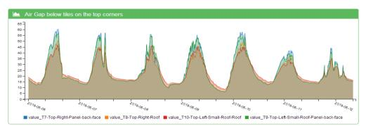
Fig. 3. Temperatures on the back side of various roofing shingle modules as well as the chassis of the roof
