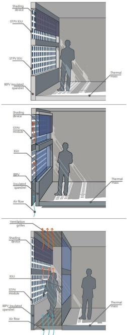
Figure 1. Schematics of the three STPV façade configurations studied: a curtain wall system incorporating STPV Insulated Glazing Units (IGU) (top), ii) STPV/T curtain wall system (middle) and iii) double skin façades incorporating STPV technologies on the outer skin (bottom).
