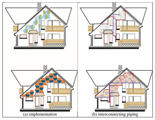
Fig. 1. Solar-thermal facades using groups of three trapeze solar-thermal collectors
