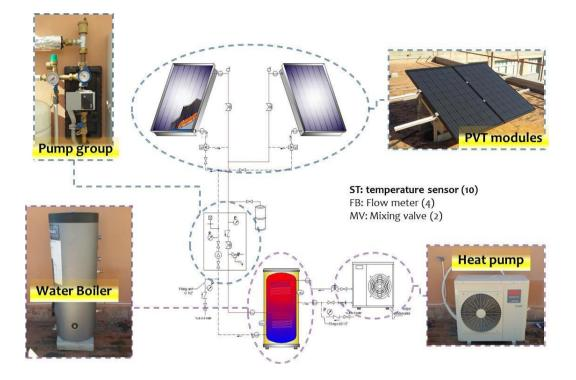
Fig. 1: PV/T power plant at the University of Catania (Italy): schematic and main components
