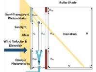
Figure 1. Sketch of the modelled DSF-P
