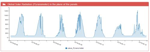
Fig. 2. Global radiation on the modules plane in Mons.
