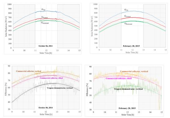
Fig. 1. Irradiance profile and efficiency of the commercial solar-thermal collectors and of the trapeze demonstrator on October 06, 2014 and February 28, 2015
