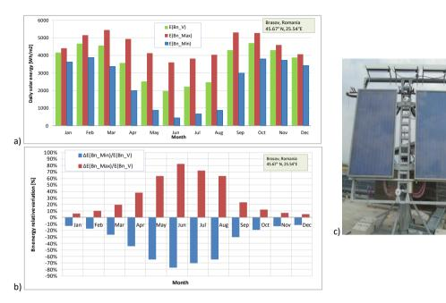
**Fig. 1:** Simulation results for a South-facing façade mounted FSTC: a) collected daily beam energy over one year in the vertical plane (V), on a plane limited oriented (± 15°) for increasing/decreasing the solar energy gain (Max/Min), b) relative variation of the collected solar energy on Max/Min oriented plane vs. fixed vertical plane V; c) experimental outdoor testing rig
