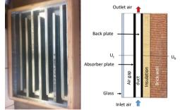
Figure 1. The modelled solar thermal collector prototype for air heating
