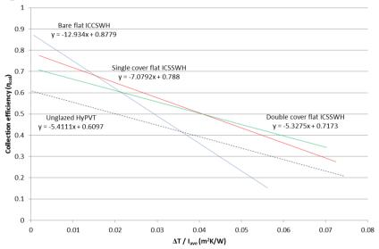
Figure 2: Collector efficiencies for the various collectors based on the absorber area and incident solar radiation of  $800 \pm 50 \text{ Wm}^{-2}$
