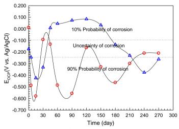
Figure 1. Open circut potentials of rebar-Ref (O) and rebar-BS (△) in 3.5% wt. NaCl solution at room temperature after 270 days immersion
