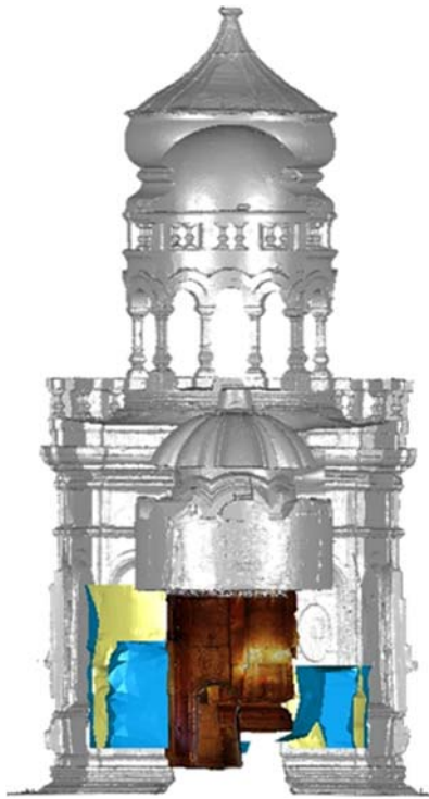
Figure 10: 3D visualization of the prospection findings: The scanned 3D model (grey) with the 3D GPR data
