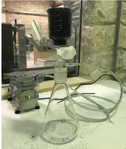
Fig. 5 Measuring the water absorption of fine lightweight aggregate
