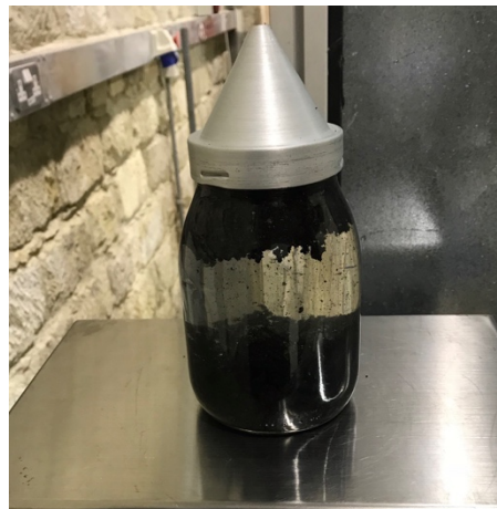
Fig. 4 Measuring the Apparent Particle Density of lightweight aggregate
