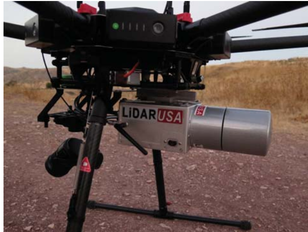
Figure 4. LiDAR HDL-32E laser scanner attached to UAV
