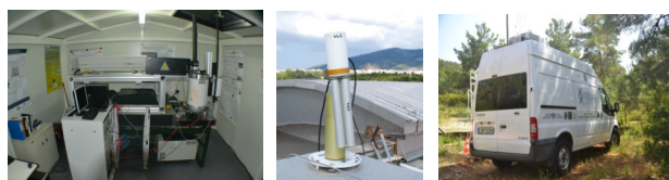
Figure 1. EOLE lidar system (left), NOA CIMEL sun photometer (middle), AIAS mobile aerosol depolarization lidar system (right).
