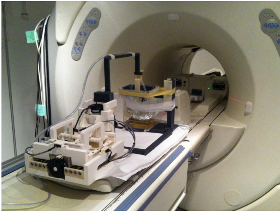
Figure 9.43: The experiment setup that was used for the evaluation of the coupling for bottom to top ultrasound delivery.
