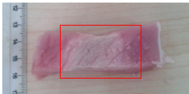
Figure 9.14: Depth of the ablation in porcine muscle with 51.4 W of acoustic power, f=2 MHz, d=5 cm, R=10 cm, duration= 8 s, focal depth=1 cm.
