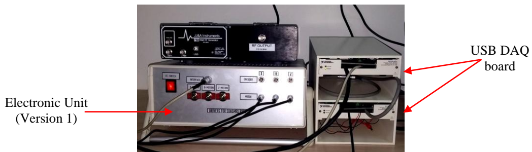
Figure 9.26: Electronics system of the positioning devices (first version).
