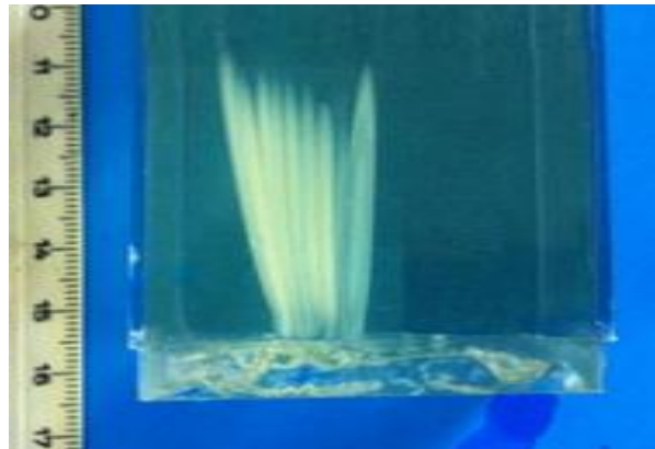
Figure 9.31: Overlapping lesions produced in gel phantom using the theta stage. Sonication parameters: Frequency at 1.18 MHz, acoustic power=45 W, duration=60 s.
